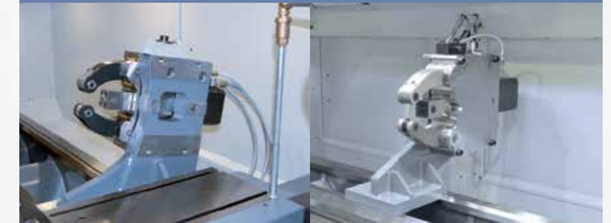
Self-centering follower rest, hydraulically actuated
