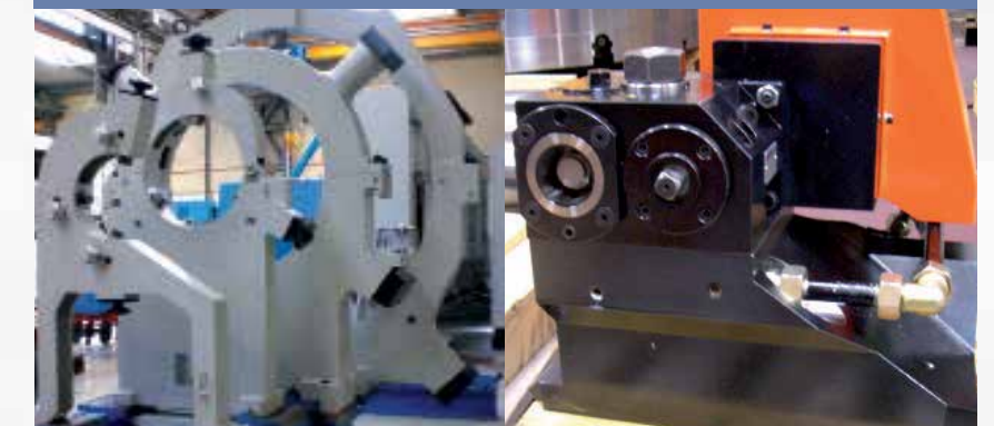
Steady rests for diameters up to 1,500 mm
