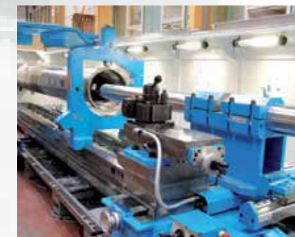
Heavy-duty boring bar holder with additional support and 160 mm bore
