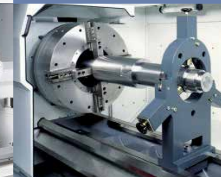
Pneumatically actuated front-end chuck with steady rest
