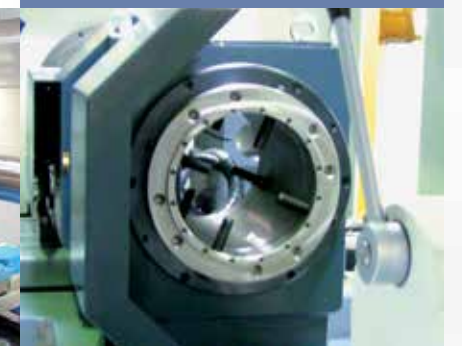
Ring steady rest with 270 mm diameter
