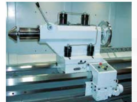
Tailstock with automated clamping and dedicated drive
