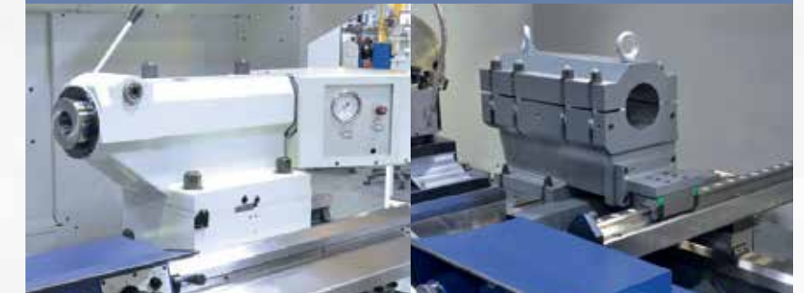
Heavy duty boring bar holder with additional support
