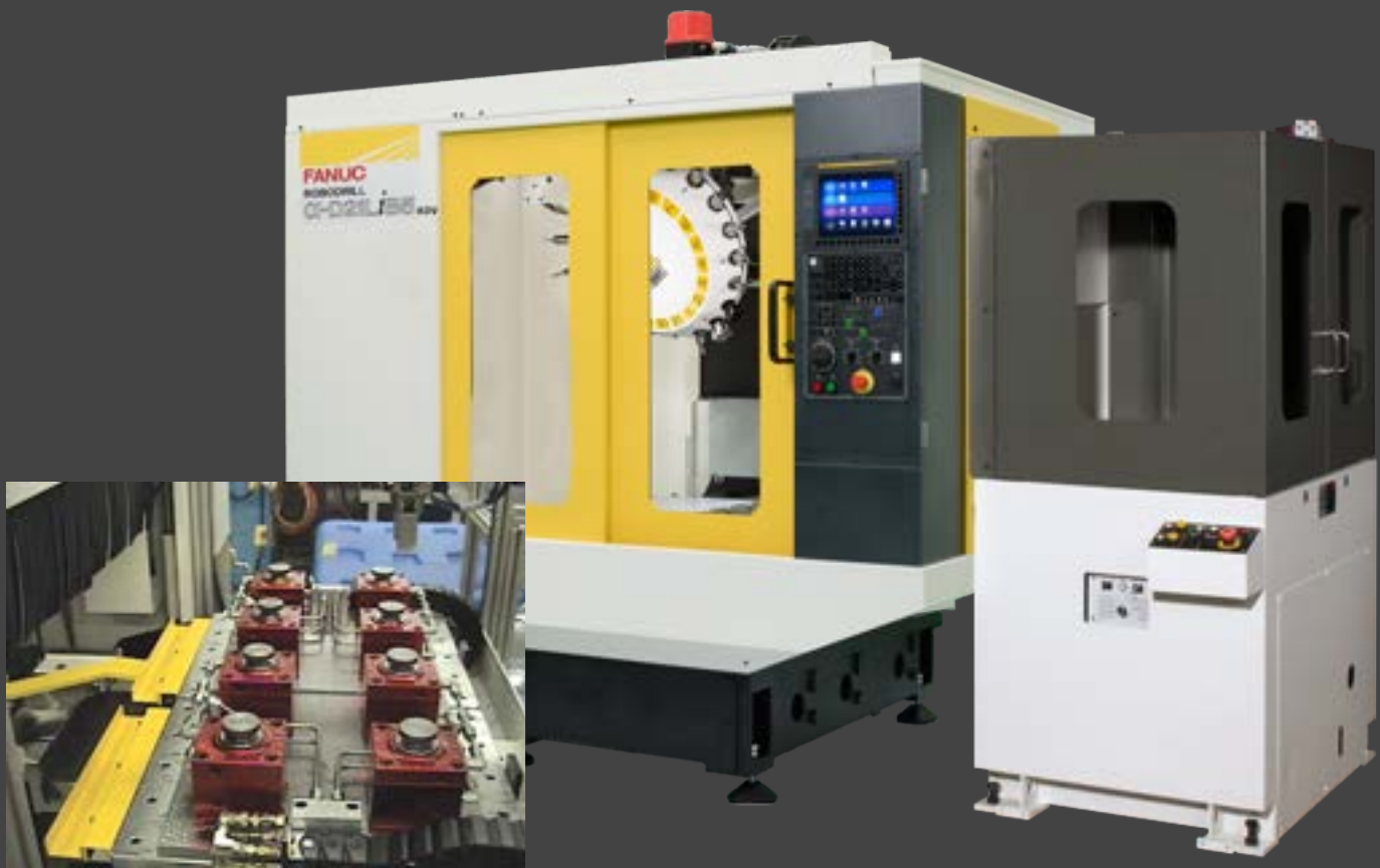
Pneumatic and Hydraulic Fixtures
