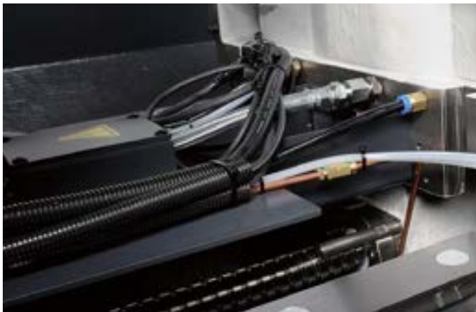
Ball screw with pre-lubricated seals
