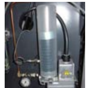
Automatic grease lubrication unit for linear guides and ball screws [Opt]
