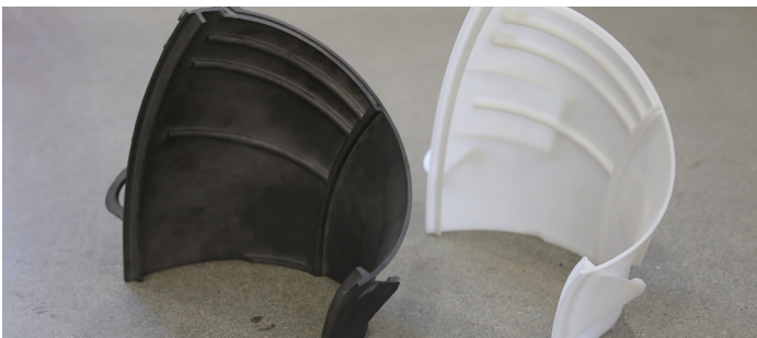
3D printed parts for Planetary Resources' Arkyd spacecraft. At left is a titanium part created by the QuickCast method on a 3D Systems SLA printer. At right is a plastic part manufactured directly by a ProJet 7000 SLA machine.
