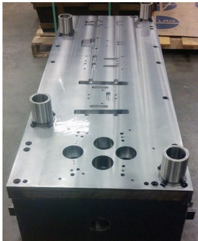
(left and above) Examples of large parts machined on the new FEELER FV-2218 Bridge Mill.
