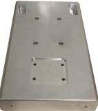
that measured 2 inches thick by 14 inches long and 8 inches wide. "To accomplish this job, we needed some large tooling as well as sufficient horsepower and spindle speed for the rapid material removal required. Using a ½-inch radius cutter, the Feeler easily machined the plates within a short cycle time with no more than 10 percent load on the spindle," Mr. Sarro says.
