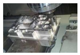
Sarro was able to leave this top plate job running 8 hours lights-out using the Feeler machine, which features an automatic power-off.
