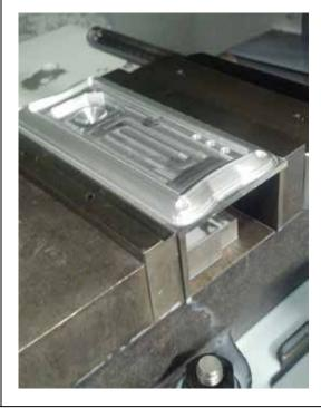
Sarro was able to machine this 0.25- by 6- by 2.5-inch face plate only after investing in the Feeler machine. It now uses the VMC along with 3D Surface Milling Technology from GibbsCAM to cut and taper the plate.
