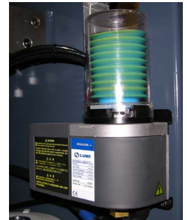
Automatic sideway lubrication system
