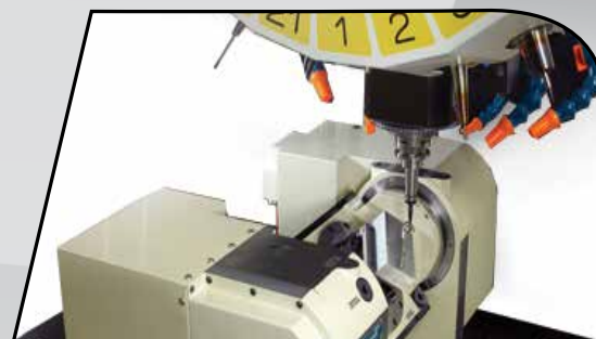
Compact integrated 5-axis table with palletized workholding
