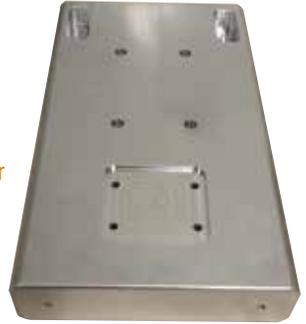
that measured 2 inches thick by 14 inches long and 8 inches wide. "To accomplish this job, we needed some large tooling as well as sufficient horsepower and spindle speed for the rapid material removal required. Using a 1/2-inch radius cutter, the Feeler easily machined the plates within a short cycle time with no more than 10 percent load on the spindle," Mr. Sarro says.
