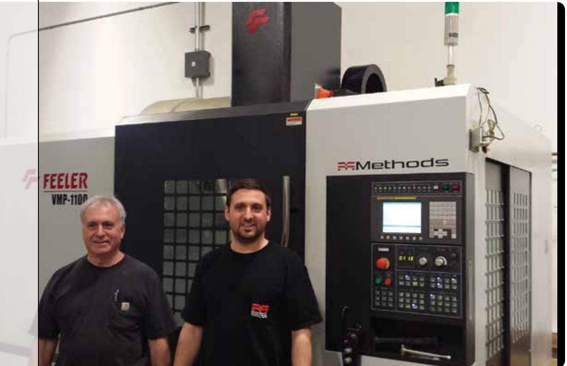
made primarily from aluminum. When the shop purchased a Feeler vertical machining center from Methods Machine Tools Inc. (Sudbury, Massachusetts), the ability to machine complete in one setup saved Sarro both time and money as well as increased productivity.
