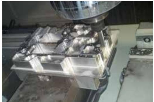
Sarro was able to leave this top plate job running 8 hours lights-out using the Feeler machine, which features an automatic power-off.
