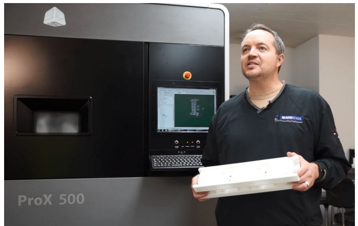
Alan Bradshaw, CEO of Idaho Steel, holds a stronger, more durable forming piston produced more than six times faster by the ProX 500 SLS printer from 3D Systems.
