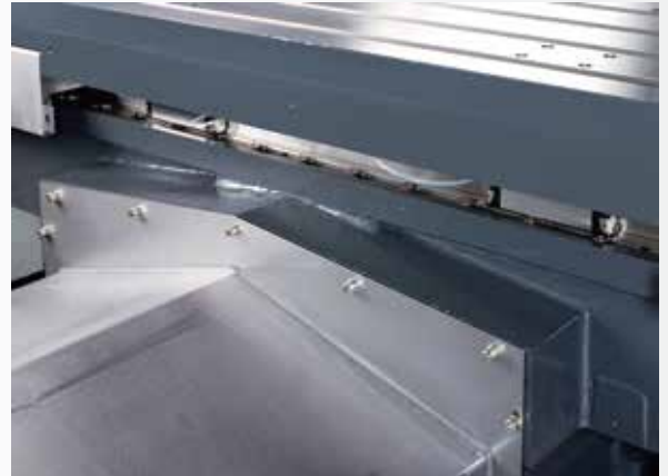
"V" shaped chip guard improves chip evacuation.
