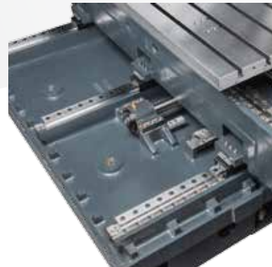
Auto Lubrication for the bearings of transmission axes
