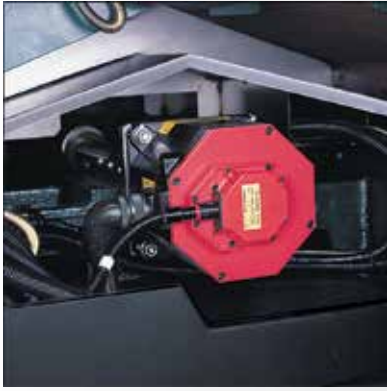
Rear installation of the Y-axis servomotor provides a convenient maintenance space.
