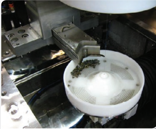
Close-up view of disk holding fixture and parts basket
