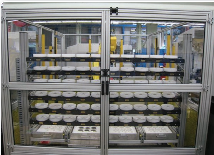
The operator station contains drawers which hold the PCD disks and a rack that holds the parts baskets
