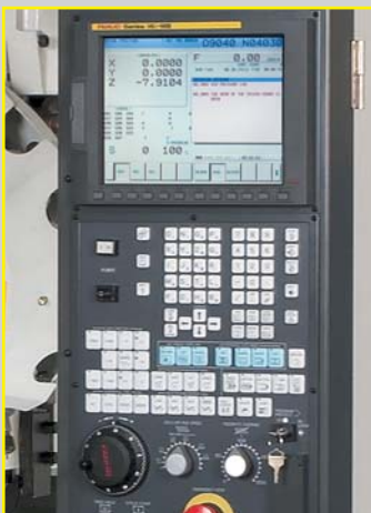
Fanuc 31-iA5 CNC with 1000 block look-ahead and block processing speed of .04 milliseconds
