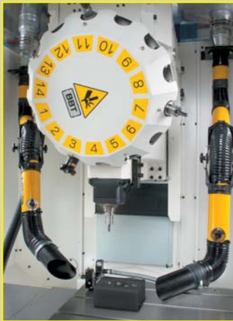
Big Plus™ 24,000 rpm spindle and 0.9-second tool changer
