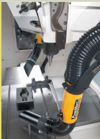
Full Torrit dust collection system
