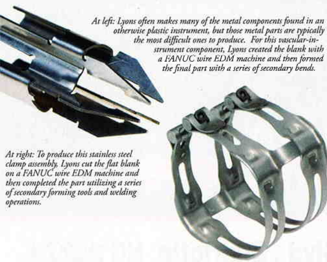
Above: The medical components Lyons produces are used in laparoscopic devices, surgical instruments, etc., approximately 80% of which are disposable. Produced in quantity from metal sheets, components such as the one shown here are first profiled on a FANUC wire EDM machine. The "fingers" are then bent and twisted.
