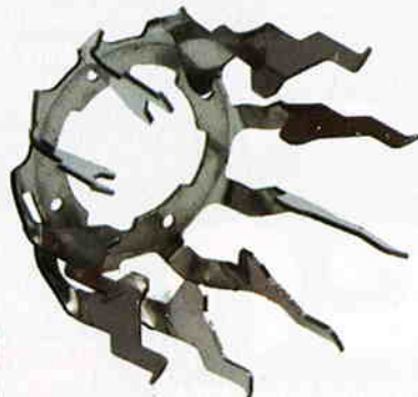
Above: The medical components Lyons produces are used in laparoscopic devices, surgical instruments, etc., approximately 80% of which are disposable. Produced in quantity from metal sheets, components such as the one shown here are first profiled on a FANUC wire EDM machine. The "fingers" are then bent and twisted.
