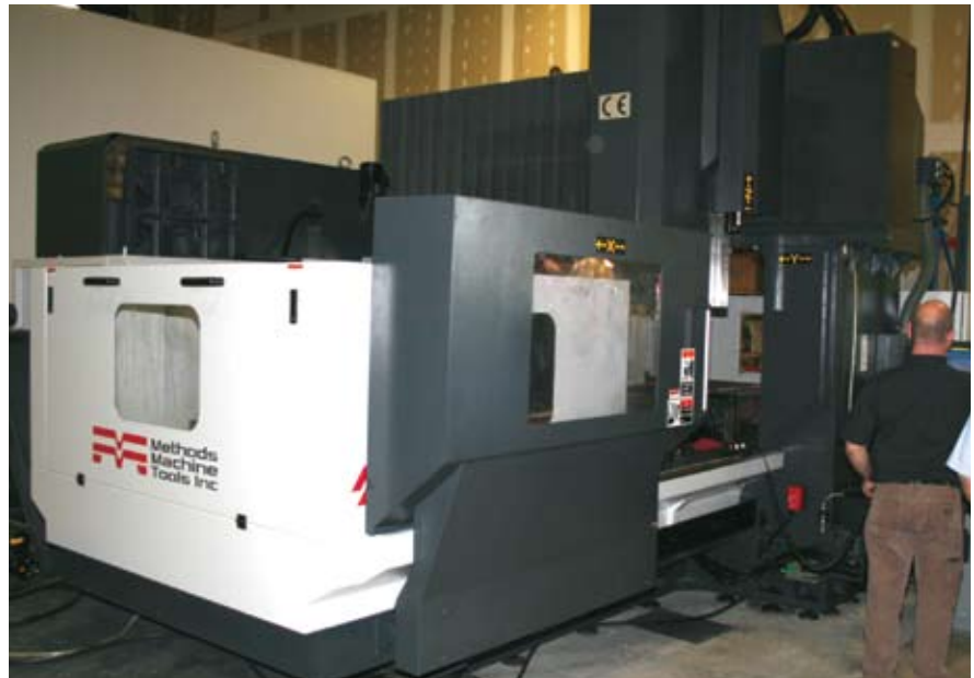
Above: Elite Tool's new Feeler FV-2218 bridge mill with capacity of 85" x 71".
