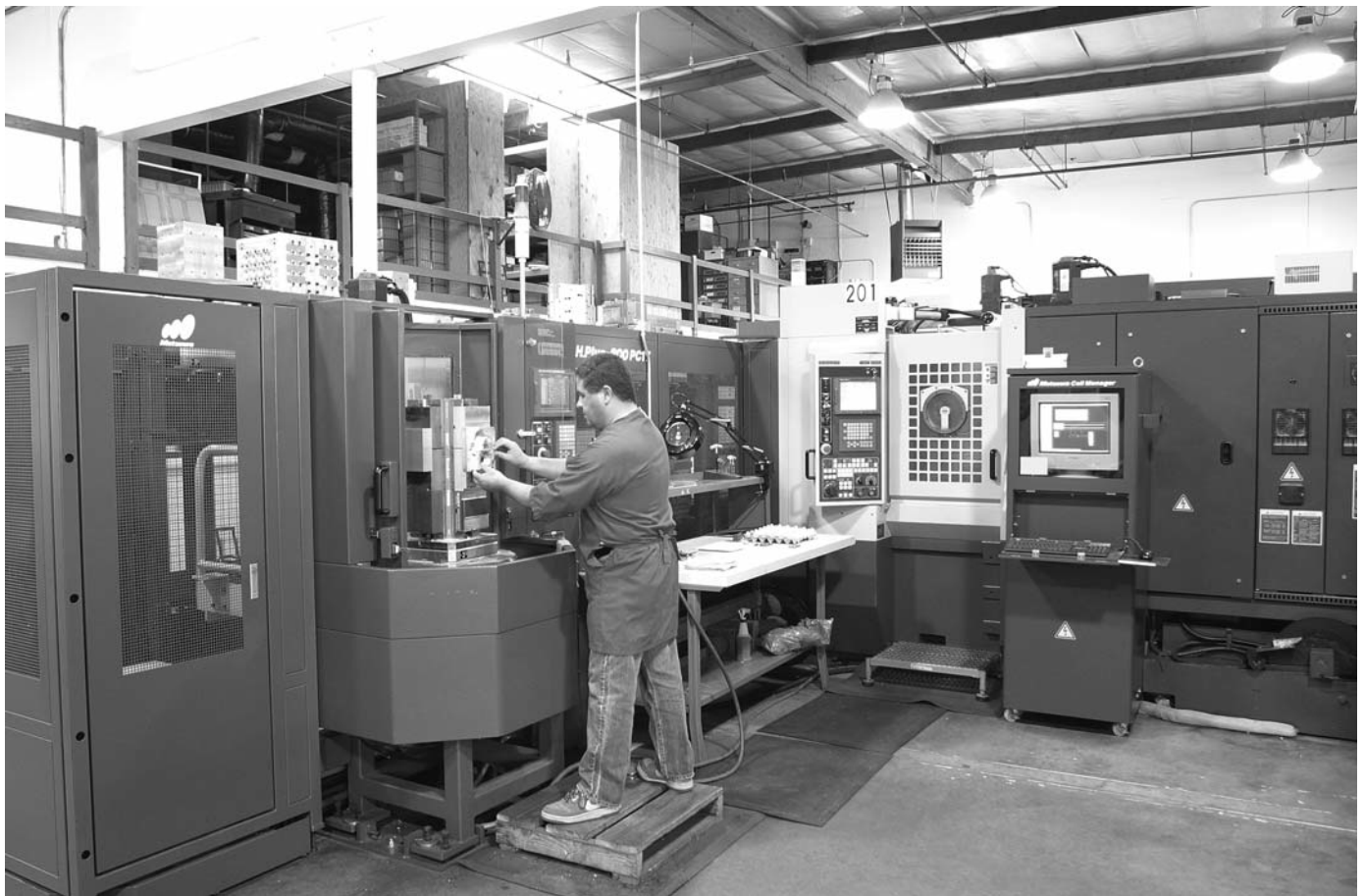
Cell operator Lawrence Rael, sets up Watts Machining's Matsuura horizontal machining center. The system is currently equipped with 12-pallet delivery and a 240-tool changer.
