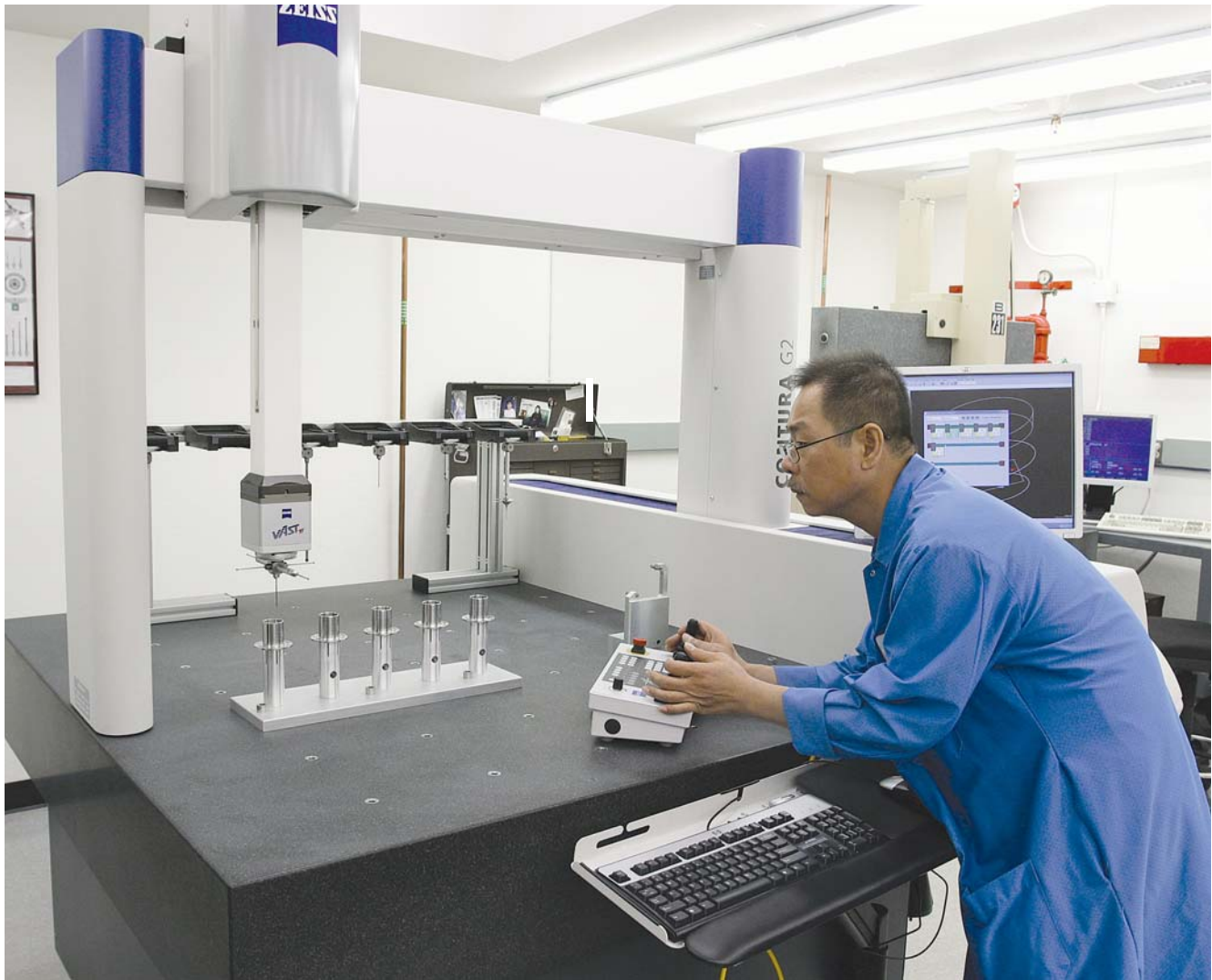
Tan Lam, Watts lead inspector, sets up the company's new Zeiss Contura G2 to inspect 5 bearings produced for Embraer. The run takes a total of 15 minutes on the Zeiss, compared to one hour for each part previously. The Zeiss is being used by Watts to pass a Measurement Systems Analysis test requested by one of the company's aerospace customers.
